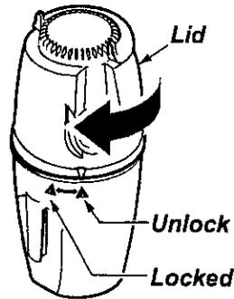
Place dust bin lid assembly back onto top of dust bin. Align marks with bin marks as shown. Rotate lid clockwise while pressing downward so that marks align as shown.
